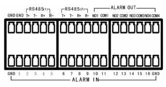
KD-402 can only be connected through "R+, R-" in 485(1) port.
